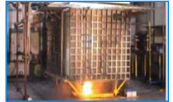
Internal Arc Tests
